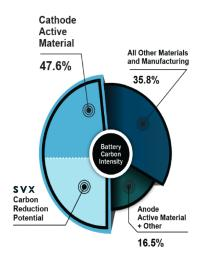
CAM also constitutes the largest carbon footprint of the lithium-ion battery and thus, the electric vehicle.
